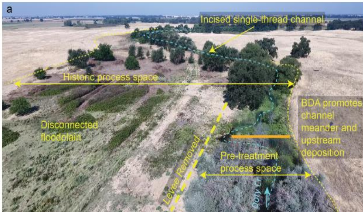
Doty Ravine Creek, California project area (a) in August 2017 before the floodplain was reconnected (b) in August 2019 after the floodplain was reconnected. Restoration design elements are highlighted on images along with gains in process space and stream recovery in response to restoration actions. Photographs: (a) Drone image by Placer Land Trust, (b) drone image by Matt Hamman.
